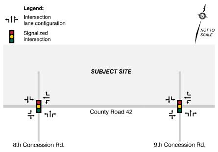
Figure 5: Assumed Intersec\(\bar{A}\)on Laning and Traffic Control
